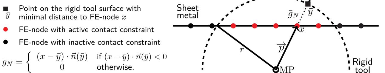
Active contact constraints add  $\frac{1}{2} \int_{\Gamma_c} \varepsilon_N (\bar{g}_N)^2 \, dA$  to the energy functional; see [6].
